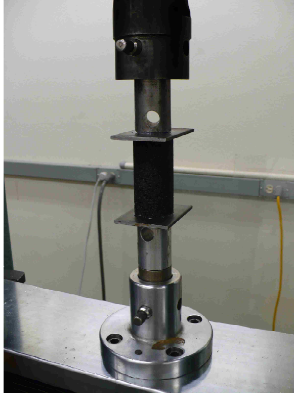
Figure 3.6 Test setup for cylindrical matrix samples
