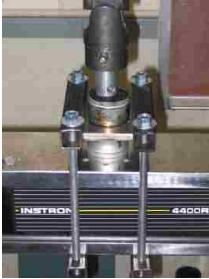
Figure 3.7 Test setup for aggregate/matrix interface in tension
